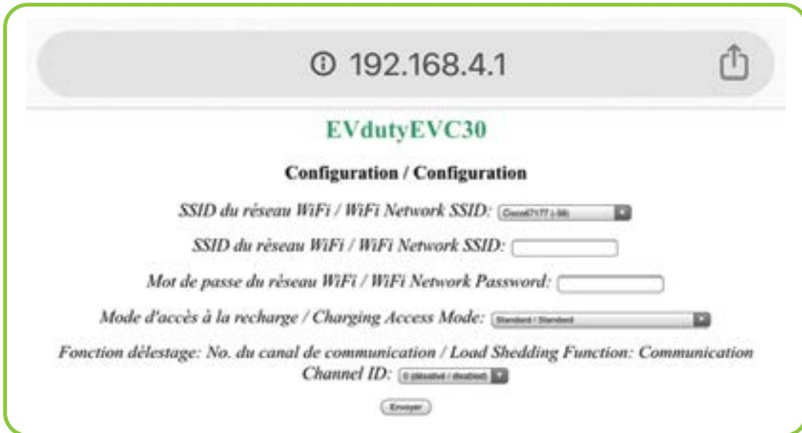
Figure 11 : Configuration borne EVC30 - Configuration
